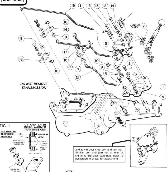
Muncie transmission is shown in the assembly drawing. Borg-Warner is recognized by curved bottom side cover shown in picture to the right. Assembly of all parts is identical to Muncie installation.
