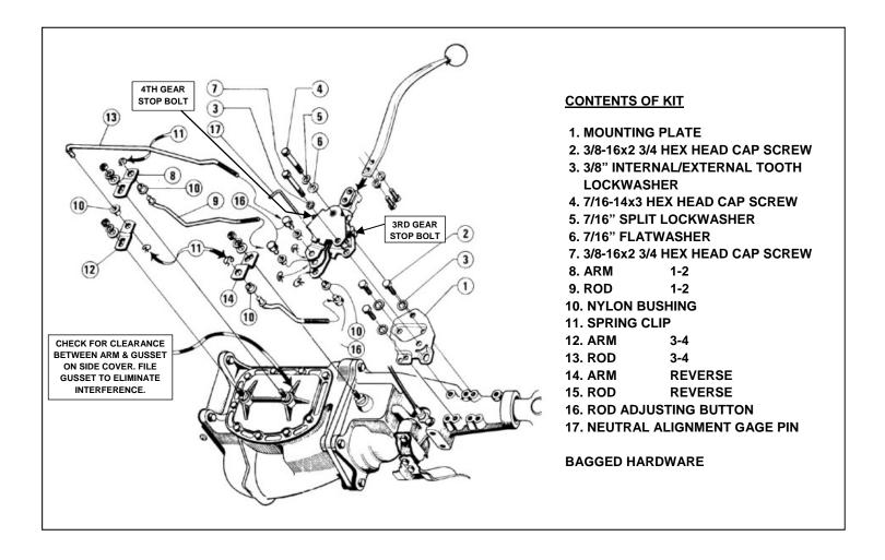
MOUNT SHIFTER IN REAR POSITION. THE RODS SUPPLIED WITH THESE KITS ARE DESIGNED FOR REAR MOUNTING.
