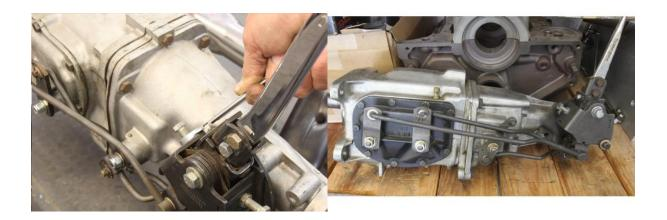
Now we can duplicate that process for Second and Fourth gears on the stop bolt on the front of the shifter. Again, loosen the stop bolt, shift into Fourth and tighten until the bolt contacts the shifter and then back out one turn and tighten the lock nut. Here is a similar Hurst Competition/Plus shifter on a Richmond Super T-10 four speed. The linkage is different but the orientation is the same as the Muncie and the adjustment procedure is also identical.
