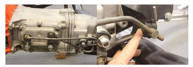
Note how the 3-4 arm angles away from the transmission case and the rod fits through with the pin pointing toward the trans. Adjust the length of the rod and then install the pin into the shifter arm and affix the spring clip.
